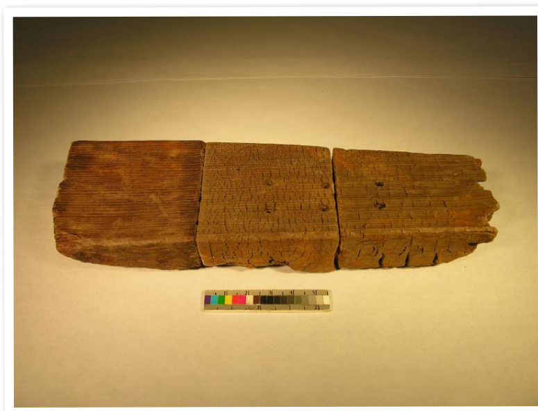
Figure 4: A piece of wood cut in three and treated three different ways. The piece on the right was dried at room temperature, the one in the centre was freeze-dried without PEG pre-treatment, and the one on the left was treated with PEG, then freeze-dried. Notice the differences of appearance and structure in the three samples. Both samples that were not treated with PEG are cracked while the one that was treated shows almost no cracks.
